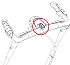
3.7. Switching off the electric lawn mower by release the lever (1) of the On/Off switch and necessarily wait for the cutting blade to stop rotating!
