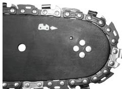
Move the guide bar (20) away from the driving chain wheel, so chain guiding links are placed in the guide bar groove.
